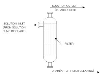
Figure 8.9 Solution purification device
