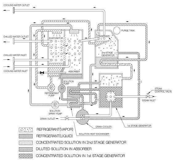
Figure 2.2.1 Cycle diagram of two stage steam absorption chiller(AR-W70~200G2)
