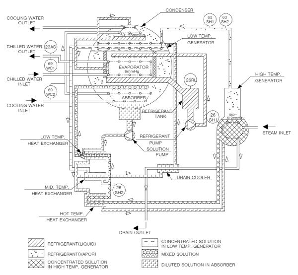
Figure 2.2.2 Cycle diagram of two stage steam absorption chiller(AR-W220~800G2)
