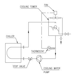
Figure 6.2 Cooling water control
