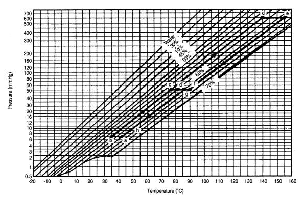
Figure 2.3 Duehring diagram with operation points
