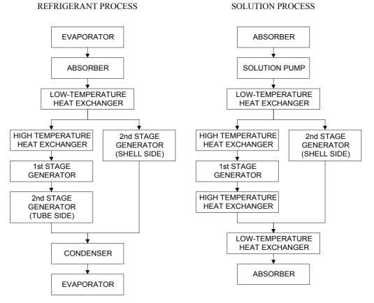
Figure 2.1 Flow diagram of solution and refrigerant
