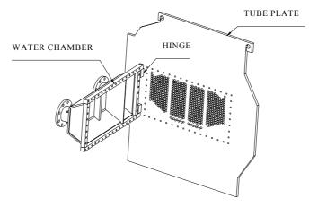
Figure 8.10.2 Opening of water chamber(AR-W220~1650G2)
