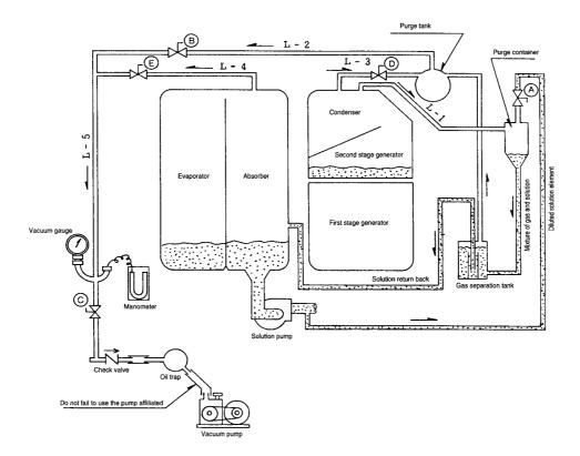
Figure 7.2.1 Purging facilities(AR-W70~200G2)
