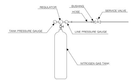
Figure 8.7 Nitrogen gas charging method
