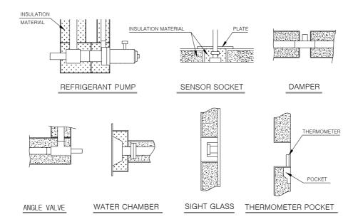
Figure 5.6 Detail drawings for insulation
