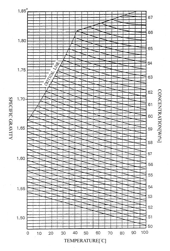
Figure 4.2 Graph for specific gravity varying with temperature and concentration
