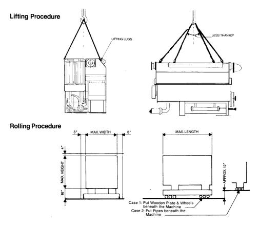
Figure 5.1.1 Rigging and moving method(AR-W70~200G2)
