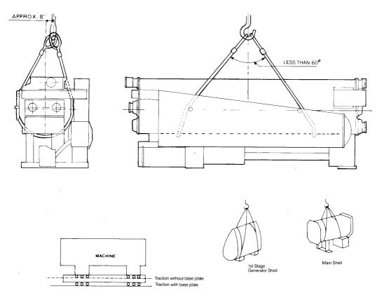
Figure 5.1.2 Rigging and moving method(AR-W220~1650G2)
