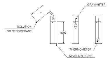
Figure 8.8 Concentration measurement method
