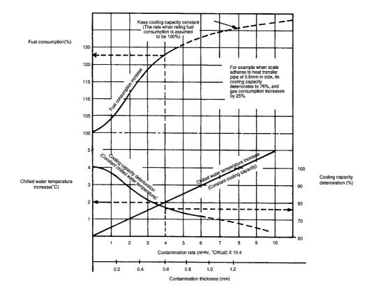
Figure 5.8 Contaminated cooling water effect on absorption chiller
