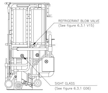
Figure 8.1.1 Facilities for refrigerant blowing(AR-W70~200G2)
