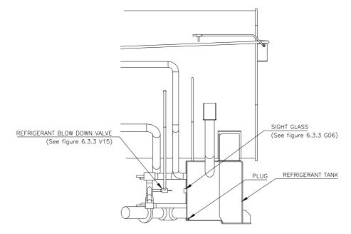
Figure 8.1.3 Facilities for refrigerant blowing(AR-W900~1650G2)
