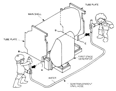
Figure 5.2 Leveling method
