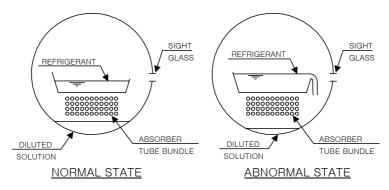
Figure 7.1.2 Refrigerant overflow schematics(AR-W220~1650G2)
