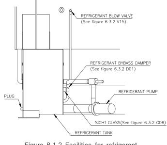
Figure 8.1.2 Facilities for refrigerant blowing(AR-W220~800G2)
