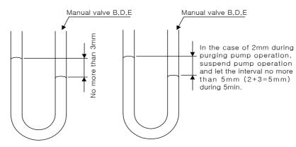
Figure 7.3 Manometer reading value after five minutes operation
