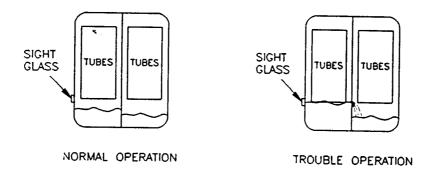
Figure 7.1.1 Refrigerant overflow schematics(AR-W80~200G2)
