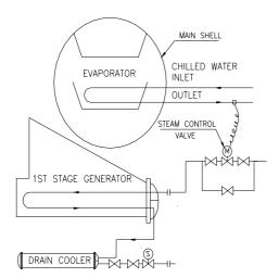
Figure 6.1 Capacity control diagram diagram
